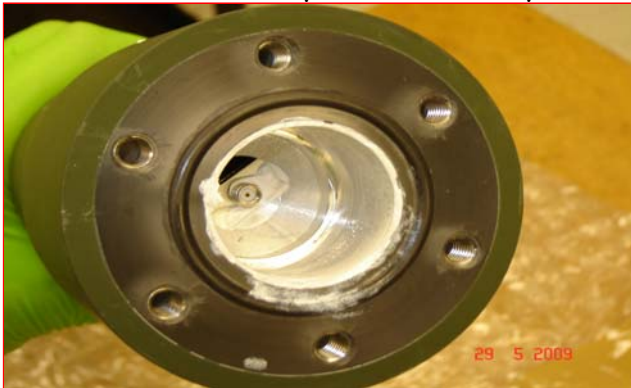
Cracks seen upon disassembly
