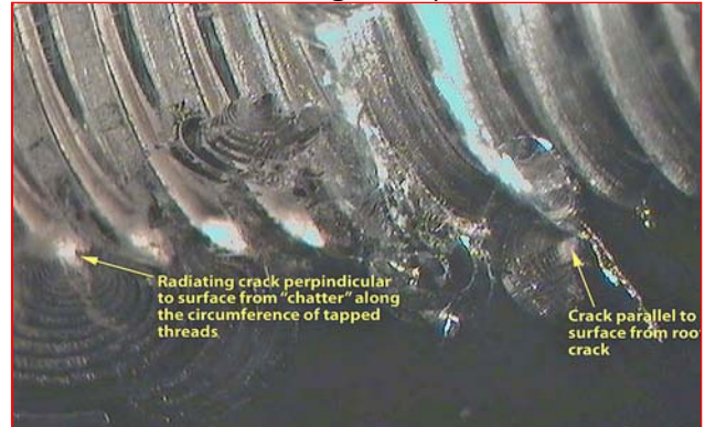
Cracks duplicated using coolant with chlorine
